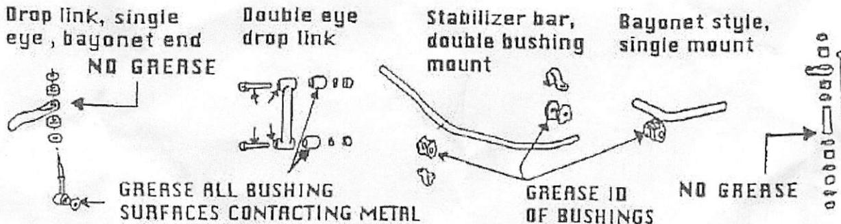
There are many types of stabilizer bars, your vehicle could have any combination of components. Lubricate your new suspension components as shown above. Lubricate track bars as you would double drop links. Use a Teflon based grease on your polyurethane components, it will give you increased performance and longevity.
