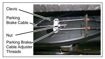
b. Pull parking brake cable through two frame mounting pads.
