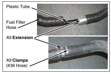
c. Install *kit* **extension** (fuel filler, metal) with two *kit* **clamps** (#36 hose).
