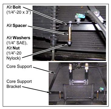
e. Adjust transmission cooler and position transmission cooler lines in factory clips.
