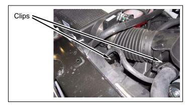
c. Tighten engine air intake hose clamps.
