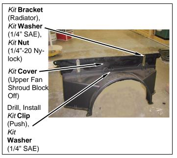
t. Install upper fan shroud assembly on core support, radiator and lower fan shroud with four bolts. Ensure kit cover (upper fan shroud block off) is placed in between core support and radiator.
