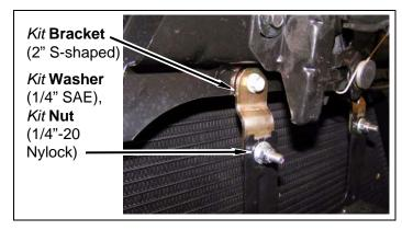
d. Install transmission cooler to core support bracket with two kit spacers (2" x .5 ID x .59 OD) with two kit bolts (1/4"-20 x 3"), four kit washers (1/4" SAE) and two kit nuts (1/4"-20 Nylock). DO NOT TIGHTEN.
