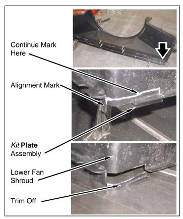
Position lower fan shroud and kit plate assembly together as marked. Using kit plate assembly as a template, drill five 1/4" holes.
