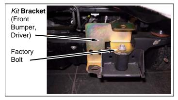
b. Install kit bracket (front bumper, inner driver) to kit bracket (front bumper, driver) and frame with three kit bolts (7/16" x 1-1/2"), six kit washers (7/16" USS) and three kit nuts (7/16" Nylock). DO NOT TIGHTEN.
