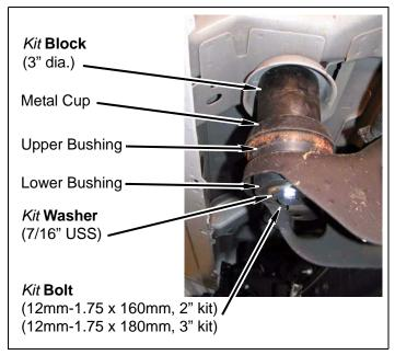
e. Install lower bushing, *kit* **bolt** (12mm-1.75 x 160mm, 2" kit **OR** x 180mm, 3" kit), *kit* **washer** (7/16" USS) on front core support cab mount. Use factory front core support cab mount nut. DO NOT TIGHTEN.
