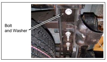
d. Remove two bolts attaching trailer hitch to bumper, if equipped.
