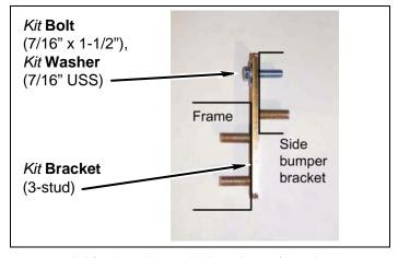
o. 3" kit: Install two kit brackets (rear bumper, 3-stud) with six kit nuts (1/2" Nylock), six kit washers (1/2" USS), two kit nuts (7/16" Nylock) and two kit washers (7/16" USS). DO NOT TIGHTEN.
