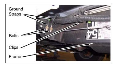
d. Remove wire clips from body and frame rail along passenger side.
