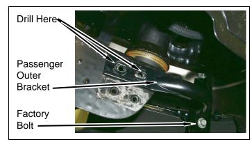
j. 2" kit: Install passenger side outer bracket to frame with two kit bolts (7/16" x 1-1/2"), four kit washers (7/16" USS) and two kit nuts (7/16" Nylock). DO NOT TIGHTEN.
