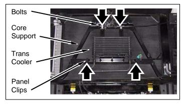
a. Remove two bolts and two panel clips attaching transmission cooler to core support.
