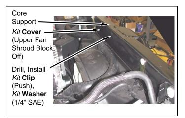
w. Check fan to fan shroud clearance. Ensure gap is uniform around shroud and tighten all nuts and bolts.
