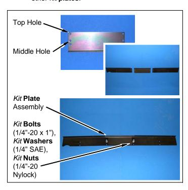
b. Install *kit* **plates** with two *kit* **bolts** (1/4"-20 x 1"), four *kit* **washers** (1/4" SAE) and two *kit* **nuts** (1/4" nylock). DO NOT TIGHTEN.
