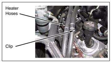
h. Install wiring harness into wire clip.
