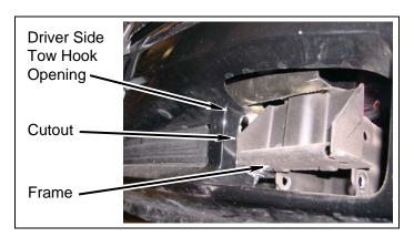
g. Install front bumper to kit brackets (front bumper) and kit brackets (front bumper, inner) with two factory bolts and nuts, and two kit bolts (7/16" x 1-1/2"), four kit washers (7/16" USS) and two kit nuts (7/16" Nylock). Apply a few drops of kit Loctite® to threads of factory bolts. DO NOT TIGHTEN.
