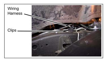
c. Install wire clips to body and frame rail along passenger side, if possible.
