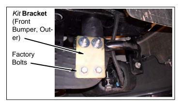
m. 3" kit: Install front outer bracket to kit bracket (front bumper, outer) with two kit bolts (7/16" x 1-1/2") four kit washers (7/16" USS) and two kit nuts (7/16" Nylock). DO NOT TIGHTEN.
