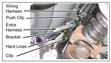
Remove two nuts and bracket from transfer case.
