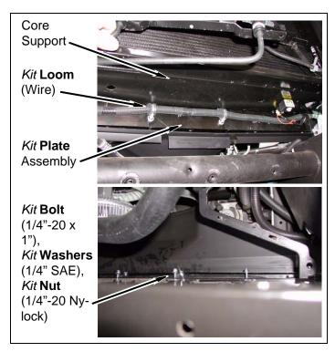
n. Install lower fan shroud on *kit* **plate** assembly with three *kit* **bolts** (1/4"-20 x 1"), six *kit* **washers** (1/4" SAE), three *kit* **nuts** (1/4" nylock) and two *kit* **clips** (push).
