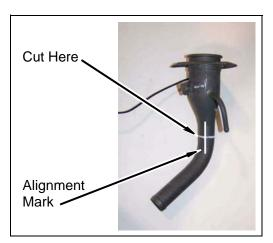
f. Deburr edges of cut ends to prevent fuel tank contamination.
