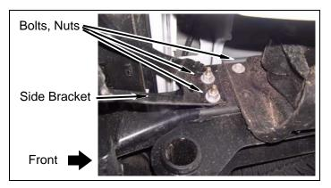
Remove two most rearward bolts attaching hitch to frame.
