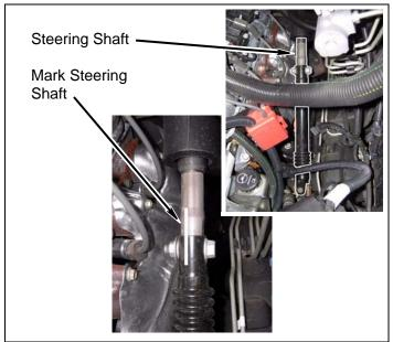
c. Remove factory bolt and nut connecting upper steering shaft to lower steering shaft.
