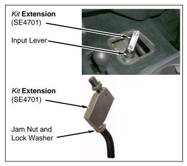
b. Install shift lever on *kit* extension. Tighten jam nut.
