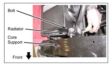
r. Assemble kit cover (upper fan shroud block off), upper fan shroud and two kit brackets (radiator) with two kit washers (1/4" SAE) and two kit nuts (1/4" nylock). s. Drill upper fan shroud using *kit* **cover** (upper fan shroud block off) as a template. Drill with a 1/4" drill bit and install a *kit* **clip** (push) as shown with a *kit* **washer** (1/4" SAE).
