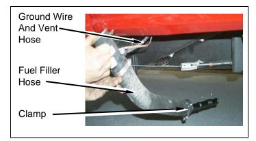
b. Carefully cut filler hose in half as shown. DO NOT CUT THROUGH PLASTIC TUBE INSIDE FILLER HOSE.
