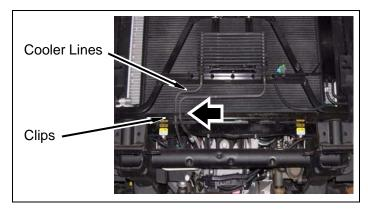
c. Remove transmission cooler from core support and allow cooler to settle on frame.
