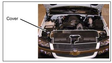
Remove six clips and grill from core support and front fenders.
