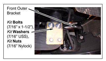
n. 3" kit: Apply a few drops of kit Loctite® to threads of factory bolt. Install front outer bracket to front bumper with factory bolt. DO NOT TIGHTEN.
