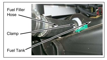
e. Install fuel filler to body with three factory bolts.
