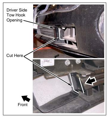
f. GMC models: Test fit bumper on vehicle and retrim bumper, if necessary.
