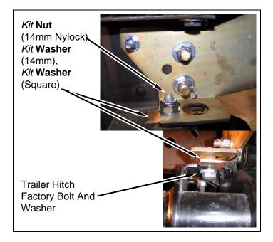
r. Place kit blocks (2" diameter, drilled) between rear bumper and trailer hitch, if equipped. Install two kit bolts (14mm-2.0 x 110mm) and two kit washers (14mm). DO NOT TIGHTEN.
