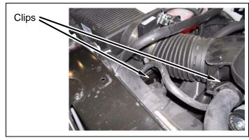
e. Remove engine air intake hose.
