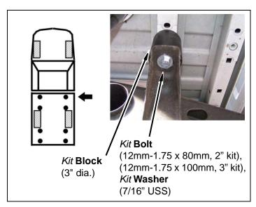
c. Place one (or two, if long bed) *kit* **block(s)** (3" diameter) on one (or two) frame mounts.
