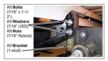
m. **2" kit:** Install two *kit* **bolts** (3/8"-16 x 1-1/2"), two *kit* **nuts** (3/8"-16 Nylock) and four *kit* **washers** (3/8" USS) to two *kit* **brackets** (rear bumper). DO NOT TIGHTEN.
