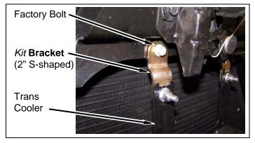
c. Install transmission cooler on two kit brackets (2" S-shaped) with kit washer (1/4" SAE) and kit nut (1/4"-20 Nylock). DO NOT TIGHTEN.
