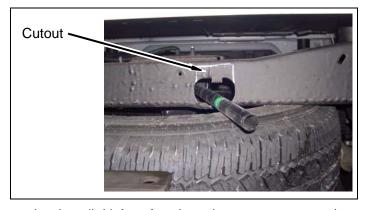
h. Install *kit* **bracket** (rear bumper, passenger) to rear bumper with factory hardware.
