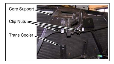
Install two kit bracket (2" S-shaped) onto clip nuts on core support with factory bolts. DO NOT TIGHTEN.
