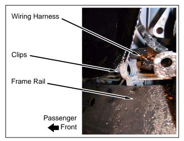
b. Install wiring harness onto brake line, if possible.
