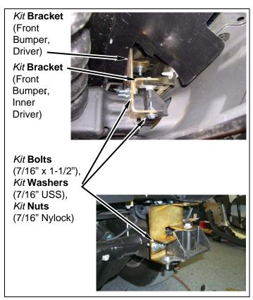
Repeat above steps for passenger side of vehicle. d. Trim driver and passenger front bumper brackets as shown.
