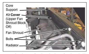
u. Attach upper fan shroud to lower fan shroud with four pop-ups on sides of fan shroud.
