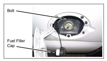
i. Install fuel filler to fuel filler hose. Adjust kit extension (fuel filler, rubber) and fuel filler hose. Tighten kit clamps (#20 hose) and fuel filler hose clamp. Install fuel filler vent hose to fuel filler and tighten vent hose clamp.
