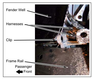
c. Remove harness clips from frame rail. Remove bolts attaching ground straps to frame.
