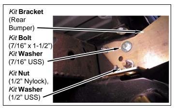
2" kit: Install kit brackets (rear bumper, 1-stud) with four kit bolts (7/16" x 1-1/2"), eight kit washers (7/16" USS) and four kit nuts (7/16" Nylock). DO NOT TIGHTEN.
