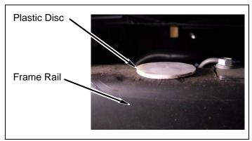
b. Install *kit* **blocks** (3" crush) in place of plastic discs with *kit* **bolt** (5/16" x 3/4" Hex head) and *kit* **washer** (5/16" USS).
