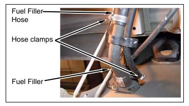
c. Remove clips securing fuel filler hose to vent hose.
